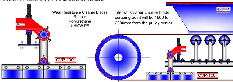
The Cleaner blades 'V' Shape opposite direction of belt travel and maintaining effective constant pressure for better cleaning. Recommended for moisturized and sticky materials. Suitable for high capacity, high speed belts with larger head pulleys. Cuts sticky material to material adhesion.
