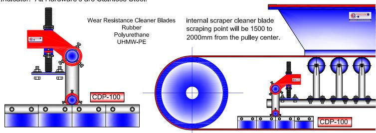
The Cleaner blades 'D' Shape opposite direction of belt travel and maintaining effective constant pressure for better cleaning. Recommended for moisturized and sticky materials. Suitable for high capacity, high speed belts with larger head pulleys. Cuts sticky material to material adhesion.
